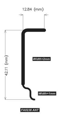
Gain: PCB antenna with maximum gain 0 dBi
