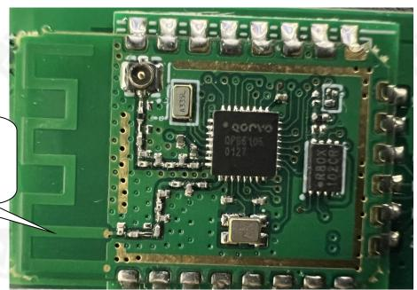
The module is designed with a PCB antenna, which the customer claims is not used and is shielded.
