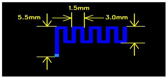
ANT operating frequency:2400MHz-2480.5MHz Max Gain: 1.33dbi ANT overall length: 41.5mm
