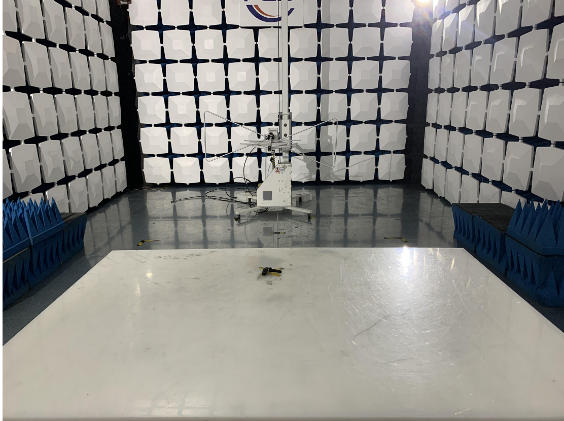
Above 1GHz for radiated emission test setup
