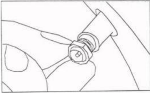
① Tighten the anti-theft nut onto the intake valve nozzle
