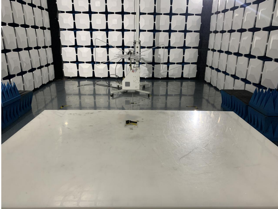
Above 1GHz for radiated emission test setup
