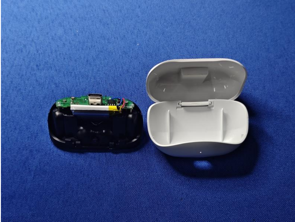
Inside View - charger base
