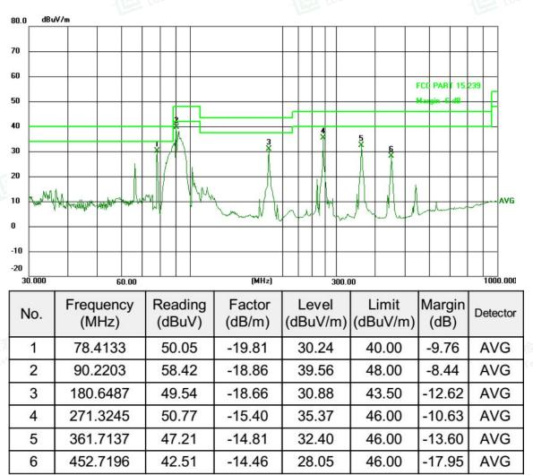
Note: The result below 30MHz and above 1GHz is too low so there is no record. The test setup show in the test setup photograph is the worst case.
