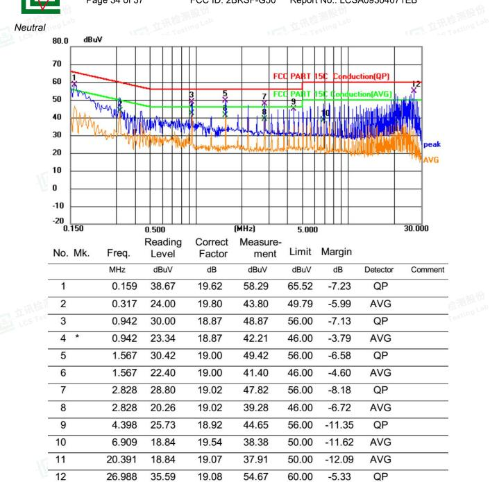
\*\*\*Note: Pre-scan all modes and recorded the worst case results in this report. Measurement = Reading + Correct Factor, Margin = Measurement – Limit, Correct Factor=Lisn Factor+Cable Factor+Insertion loss of Pulse Limiter.
