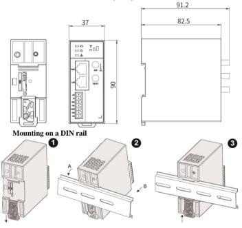
1. Pull down the DIN rail mounting hook at the back of the module.
