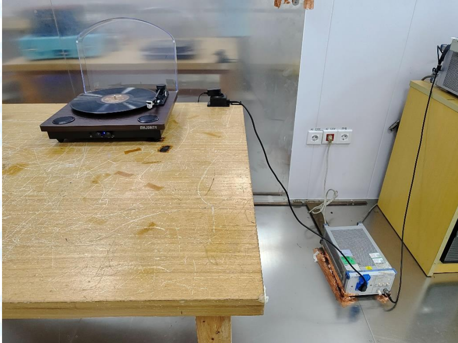
Photo of Setup for Radiated Emission (30MHz~1GHz)
