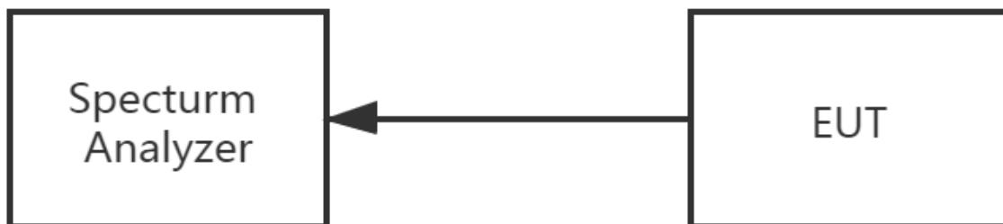
The EUT which is powered by the \${ POWER BY}, is connected to the Spectrum Analyzer; the RF load attached to the EUT antenna terminal is 50 Ohm; the path loss as the factor is calibrated to correct the reading. Make the measurement with the spectrum analyzer's resolution bandwidth(RBW) = 100 kHz. In order to make an accurate measurement, set the span greater than RBW.
