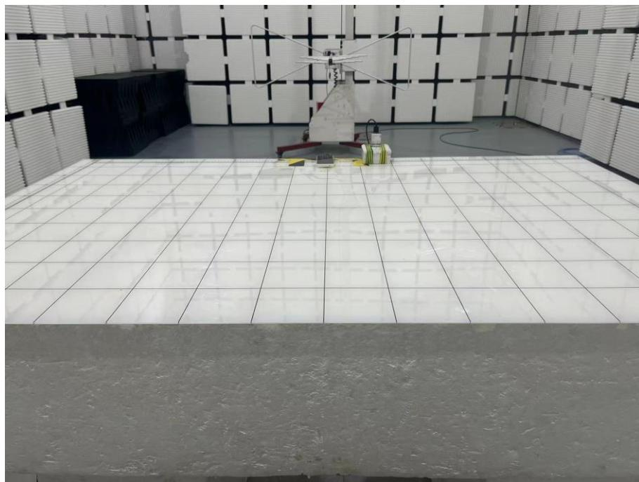
**Set-up for Radiated Emission (RE), Above 1GHz**
