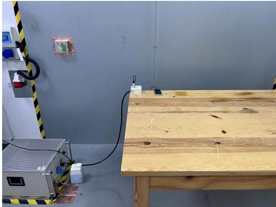
**Set-up for Radiated Emission (RE), Below 1GHz**
