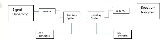
Figure 3-2 Test Setup for Conducted Measurement Radar Verification
