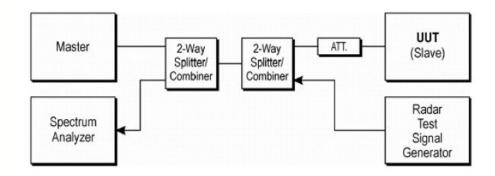
Figure 3-1. Conducted Test Setup for DFS
