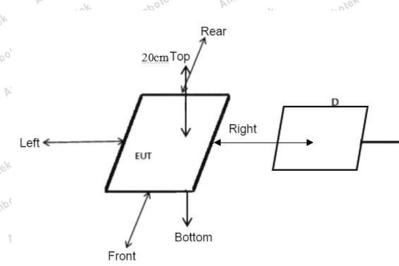
Note: Measurements should be made at 20 cm surrounding the EUT and 20cm above the top surface of the EUT.
