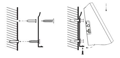
3 Fix the device on the backplate and fix the bottom screw.
