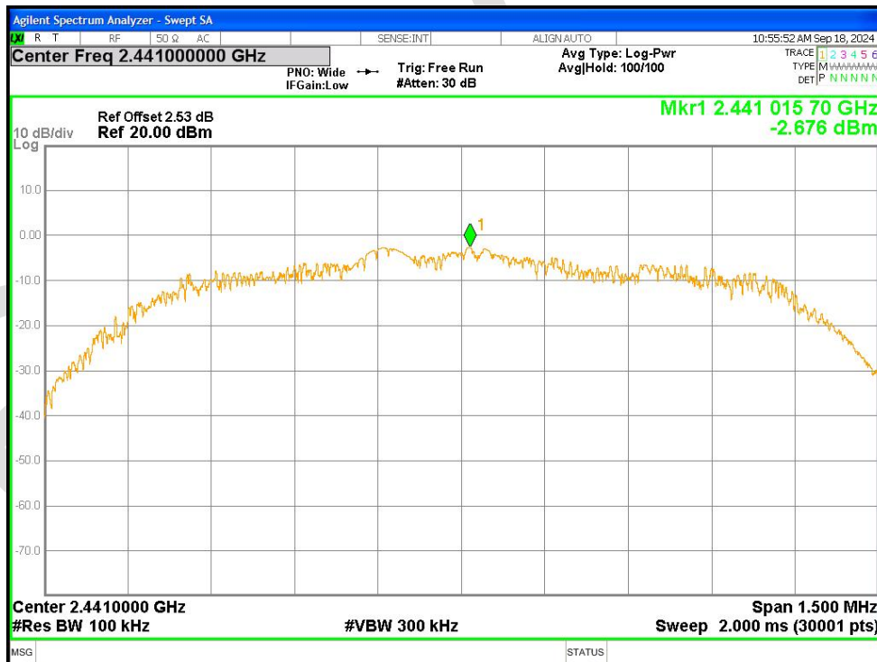
Tx. Spurious NVNT 3-DH1 2441MHz Ant1 Emission
