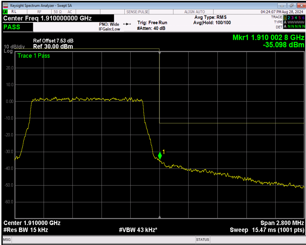
Band2 QPSK BW=5MHz Channel=18625 RB Size=1 Position=#0
