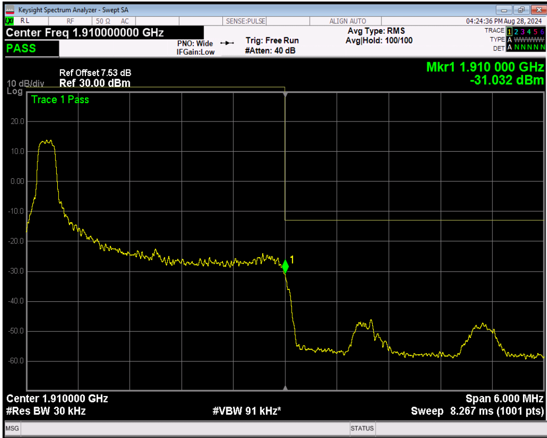
Band2 16QAM BW=3MHz Channel=19185 RB Size=1 Position=#Max
