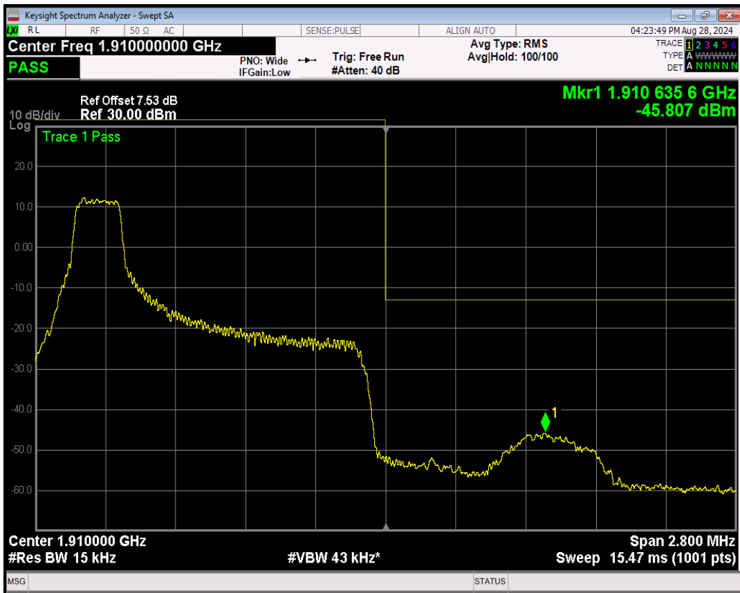
Band2 QPSK BW=1.4MHz Channel=19193 RB Size=1 Position=#Max
