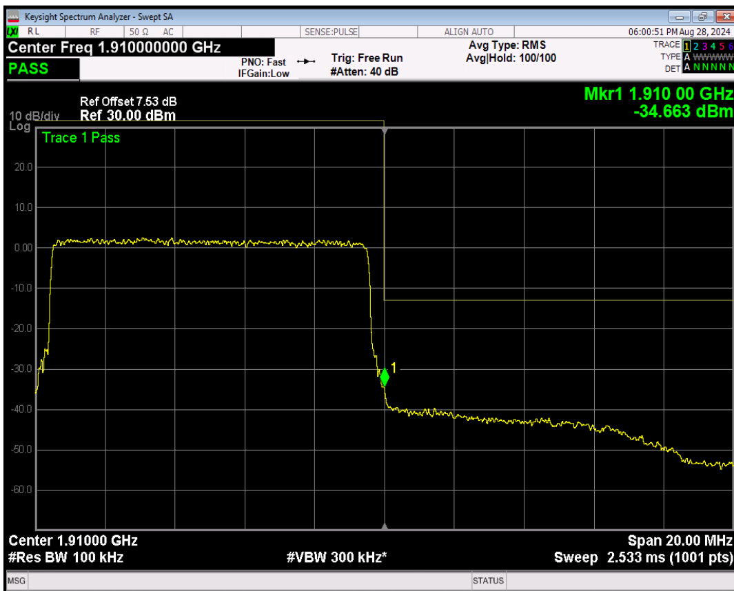
Band2 16QAM BW=10MHz Channel=19150 RB Size=1 Position=#0
