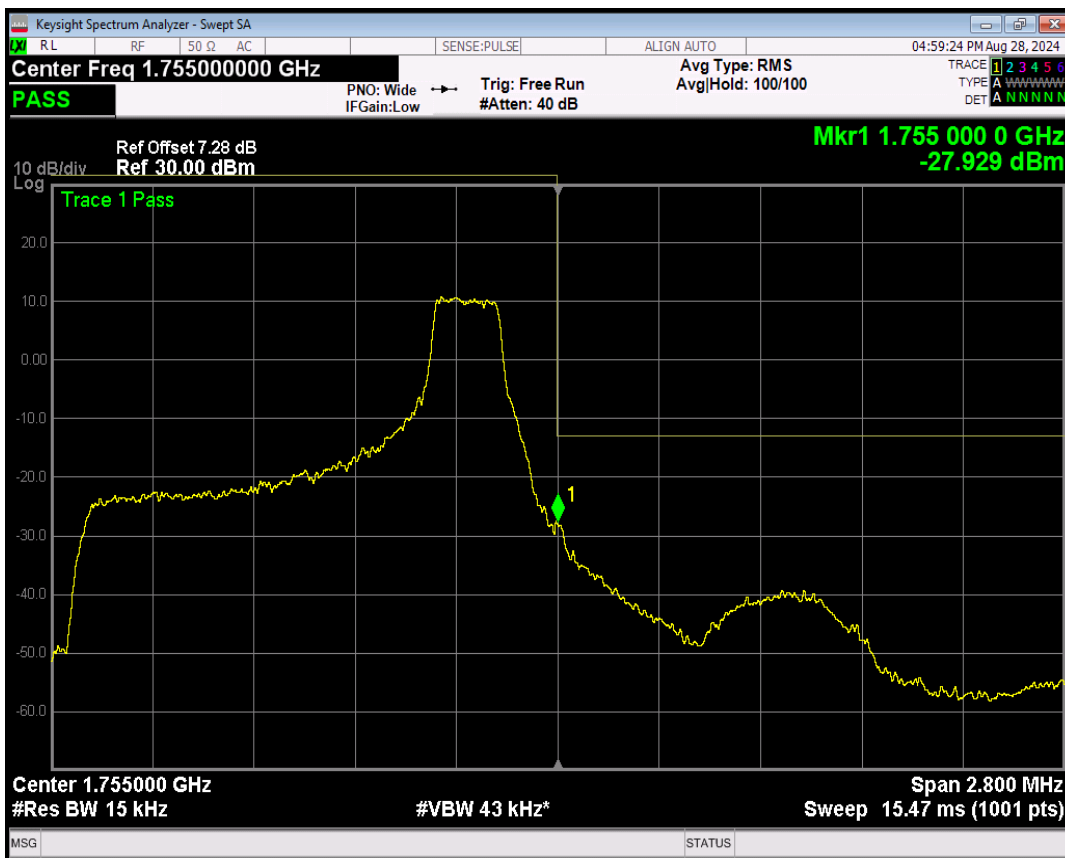
Band4 16QAM BW=1.4MHz Channel=20393 RB Size=6 Position=#0
