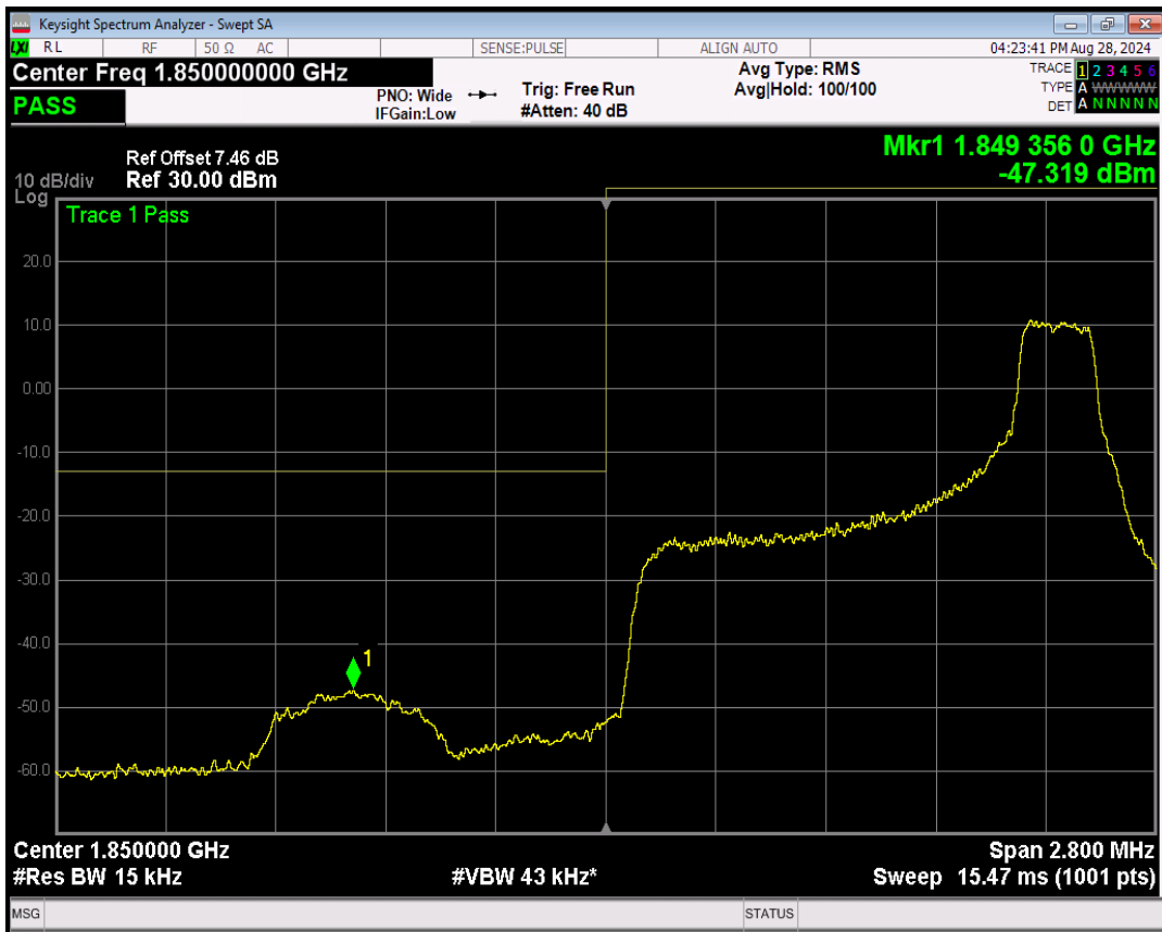
Band2 16QAM BW=1.4MHz Channel=18607 RB Size=6 Position=#0
