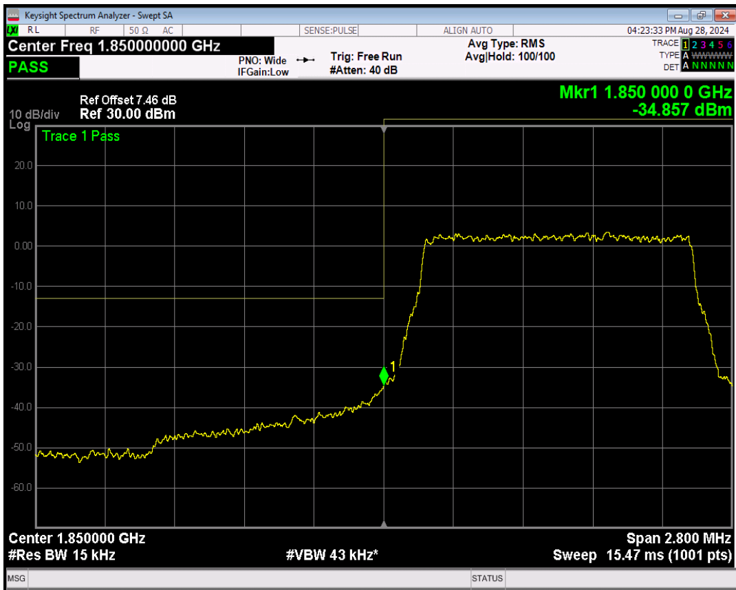
Band2 16QAM BW=1.4MHz Channel=18607 RB Size=1 Position=#0
