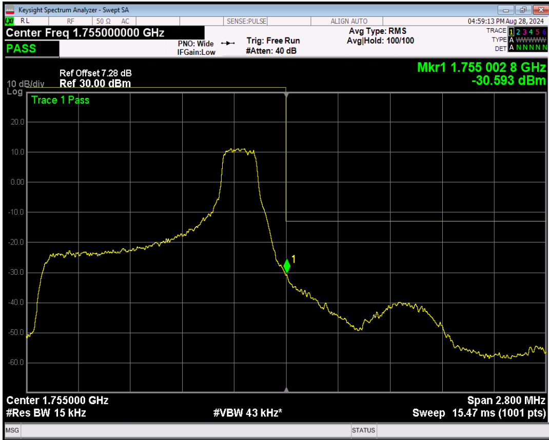
Band4 QPSK BW=1.4MHz Channel=20393 RB Size=6 Position=#0
