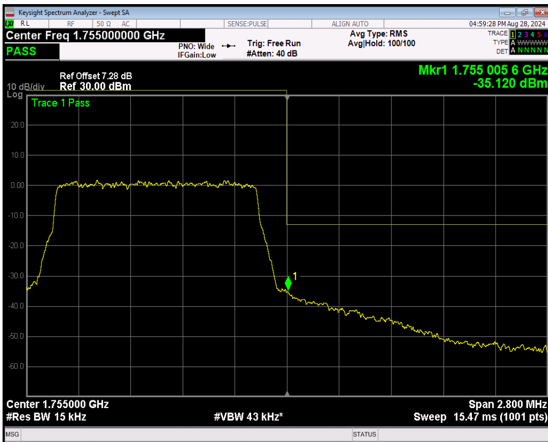
Band4 QPSK BW=5MHz Channel=19975 RB Size=1 Position=#0
