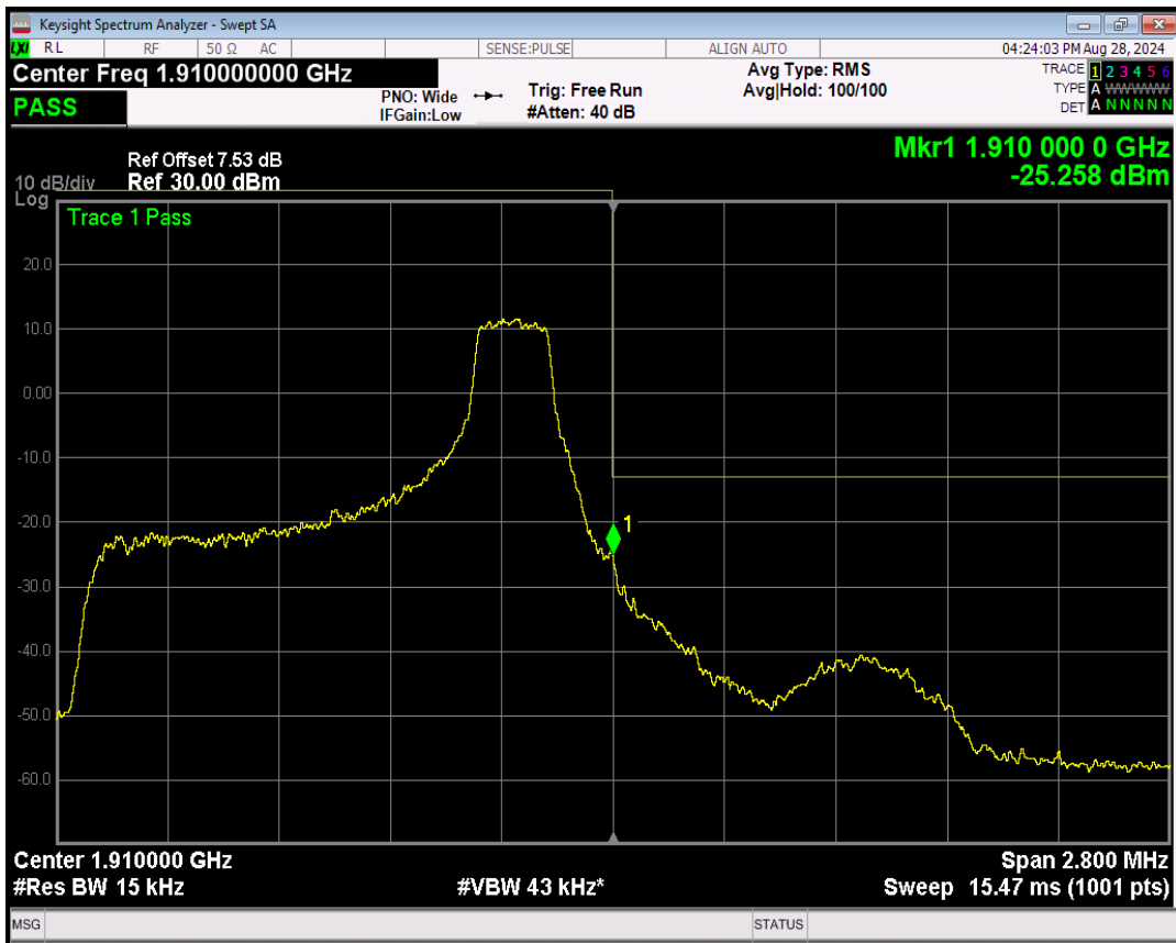
Band2 16QAM BW=1.4MHz Channel=19193 RB Size=6 Position=#0
