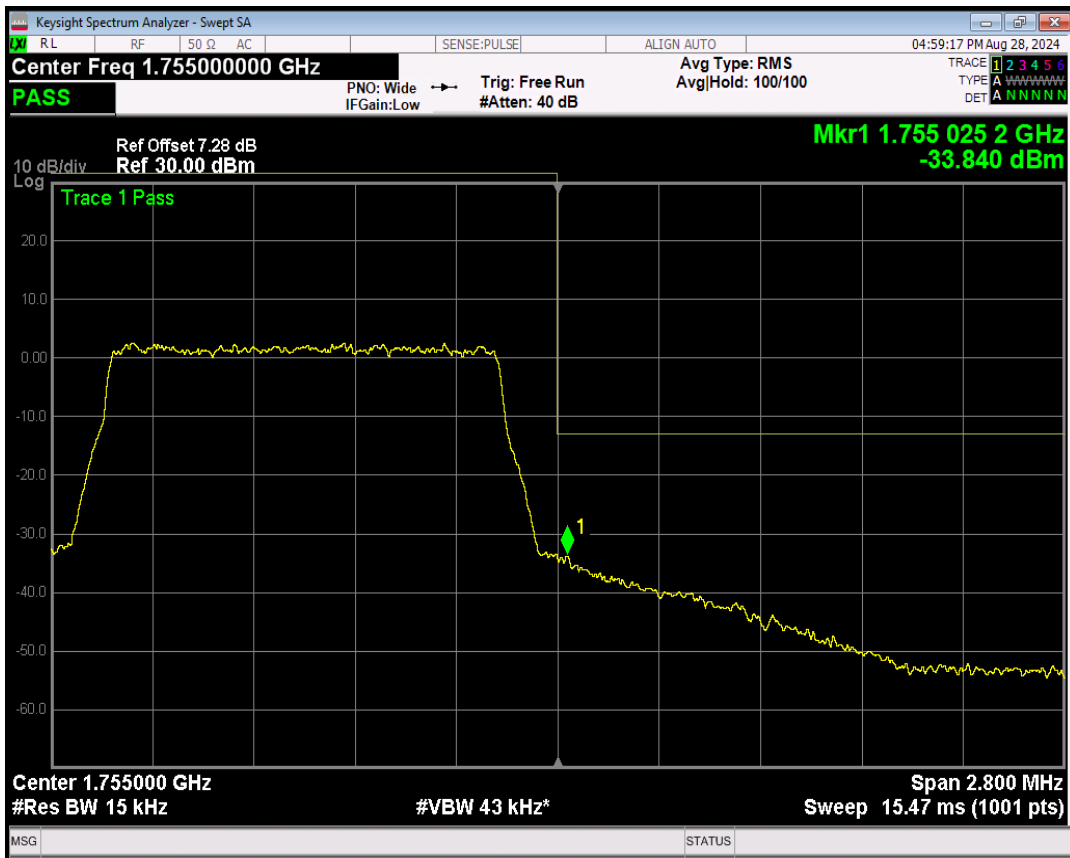
Band4 16QAM BW=1.4MHz Channel=20393 RB Size=1 Position=#0
