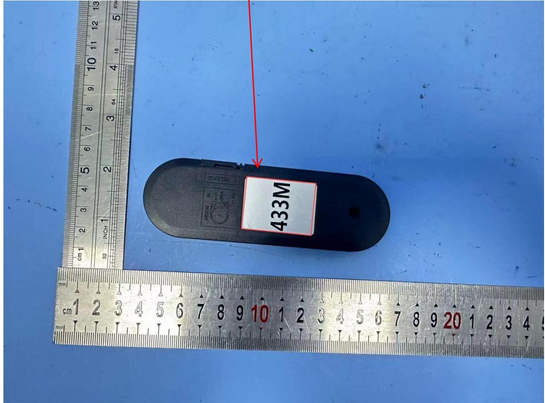
Note: The label is printed on the product by means of Spray paint.
