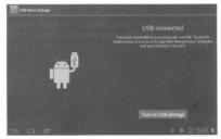
Into the load mode, you can copy, delete the file on thedevice and the file on the memory card.
