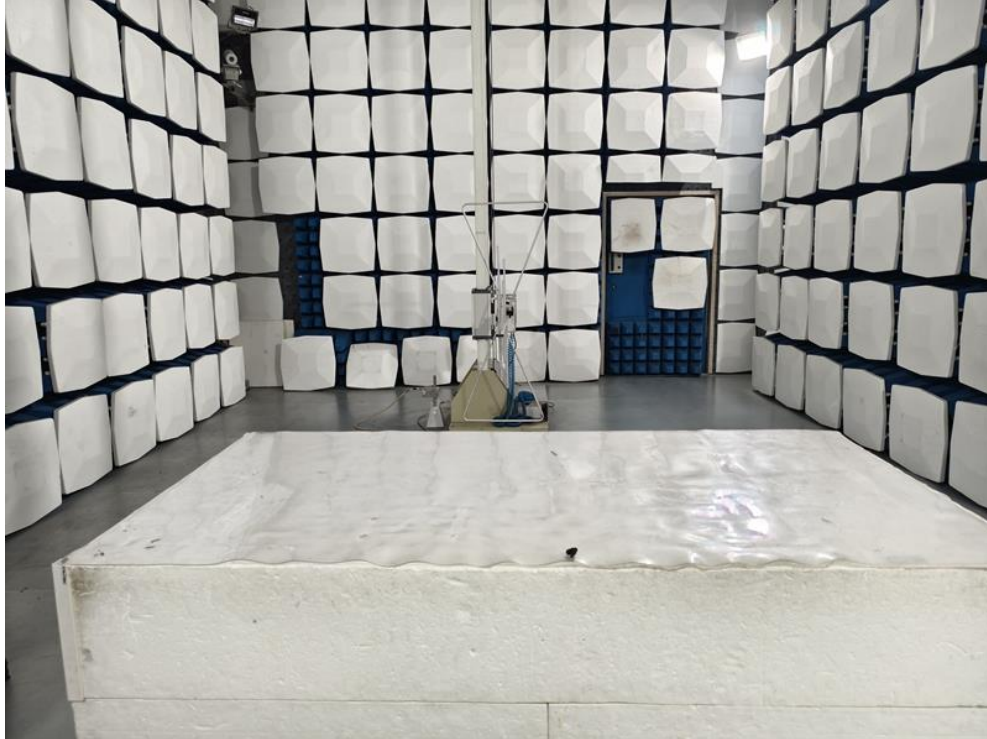
Radiated Emission Test Setup:
