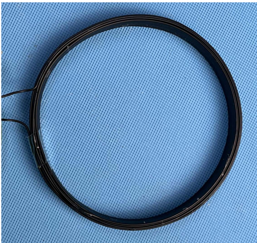
The antenna is air coil made up of 50 turns of 7/0.2mm wire and has a outer diameter of 122mm.
