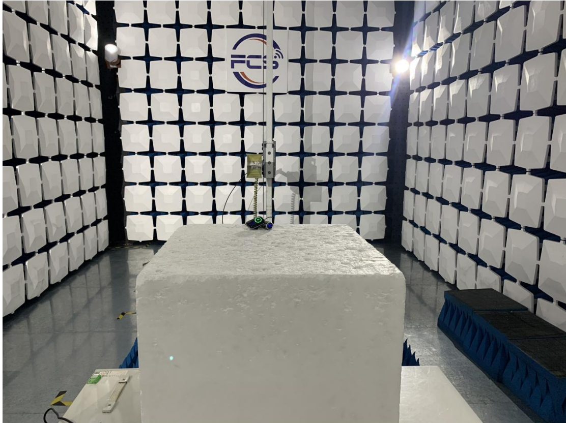
Above 1GHz for radiated emission test setup
