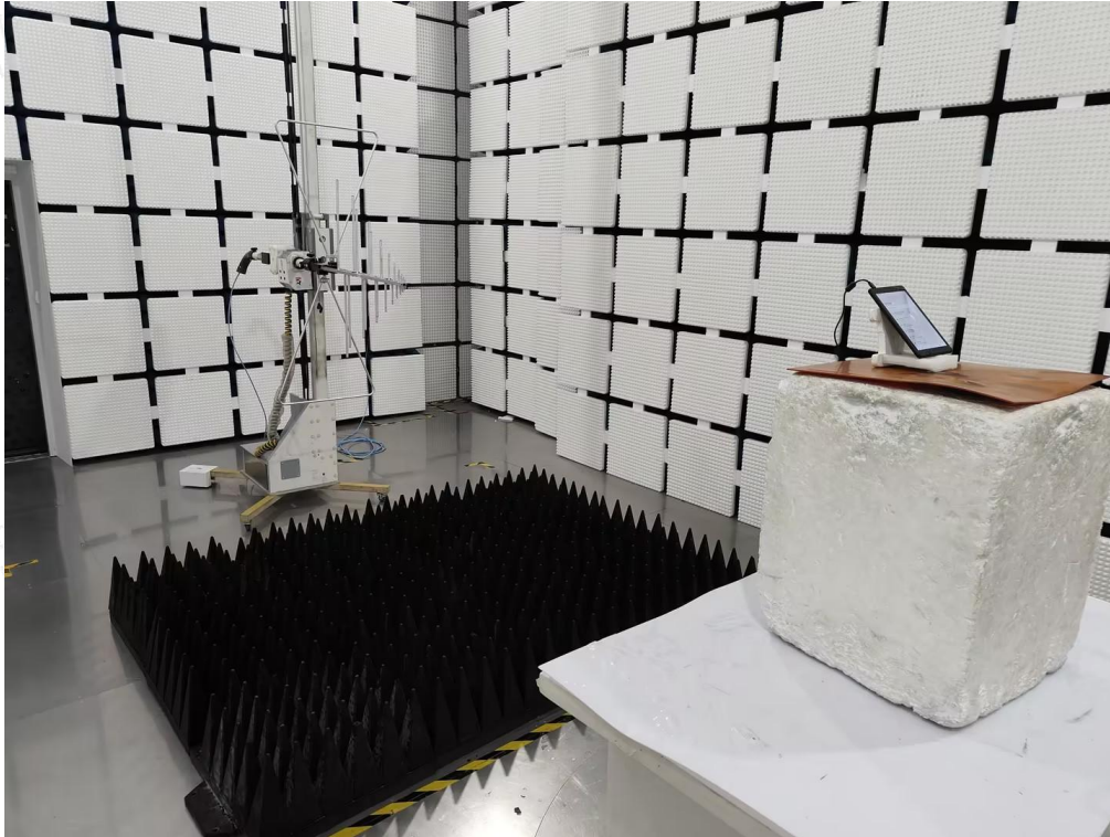
Radiated Emissions Measurement (Below 1GHz)
