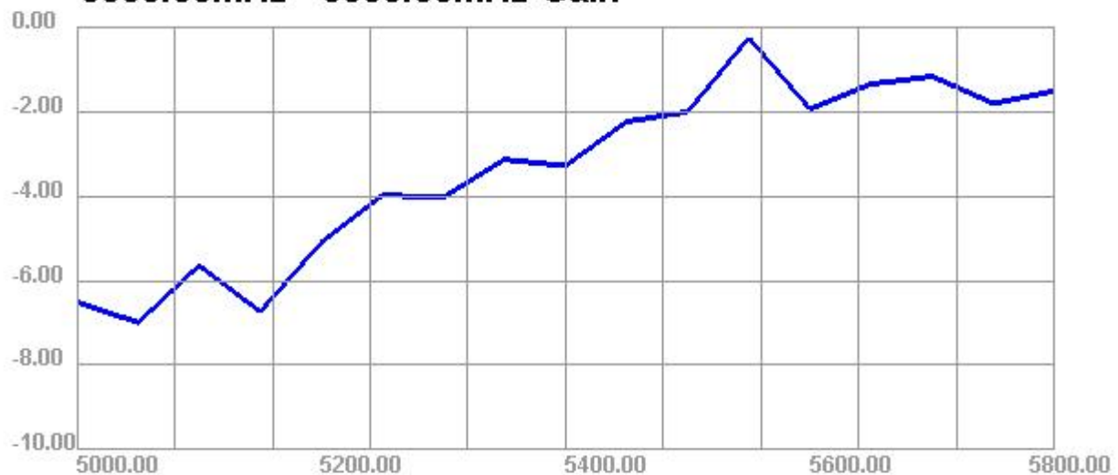
Passive Test For 5.8 Freq (MHz) Effi (%) Effi (dB) Gain (dBi) Gain (dBd) UHS (%) DHS (%) Max (dB) Min (dB) 5000 7.74 -11.11 -6.5 -8.65 4.061 3.681 -6.5 -22.06 5050 7.99 -10.98 -6.99 -9.14 4.281 3.706 -6.99 -22.24 5100 8.93 -10.49 -5.64 -7.79 5.063 3.864 -5.64 -21.76 5150 8.17 -10.88 -6.73 -8.88 4.499 3.672 -6.73 -21.32 5200 10.88 -9.63 -5.09 -7.24 5.86 5.019 -5.09 -21.72 5250 12.54 -9.02 -3.98 -6.13 7.446 5.093 -3.98 -24.47 5300 14.42 -8.41 -4.02 -6.17 8.749 5.666 -4.02 -18.34 5350 14.74 -8.31 -3.13 -5.28 8.646 6.096 -3.13 -21.94 5400 17.24 -7.64 -3.28 -5.43 9.748 7.49 -3.28 -16.48 5450 20.27 -6.93 -2.24 -4.39 11.535 8.735 -2.24 -14.96 5500 22.9 -6.4 -2 -4.15 12.381 10.52 -2 -13.89 5550 25.75 -5.89 -0.25 -2.4 13.794 11.957 -0.25 -17.38 5600 25.61 -5.92 -1.94 -4.09 13.324 12.281 -1.94 -19.73 5650 25.97 -5.85 -1.35 -3.5 12.984 12.988 -1.35 -20.28 5700 29.57 -5.29 -1.17 -3.32 14.961 14.607 -1.17 -22.27 5750 29.06 -5.37 -1.81 -3.96 14.958 14.099 -1.81 -18.72 5800 27.88 -5.55 -1.51 -3.66 14.688 13.196 -1.51 -16.4
