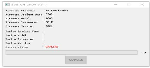
2. Press the left 3D in the hibernation state of the controller to keep it (note that this operation can not be accidentally touch other buttons to wake up the controller), use the TYPE-C cable to connect the controller to the PC, connect well and release the left 3D, at this time "DOWNLOAD" from gray to black, that is, the connection is successful, click Click "DOWNLOAD" to upgrade, as follows:
