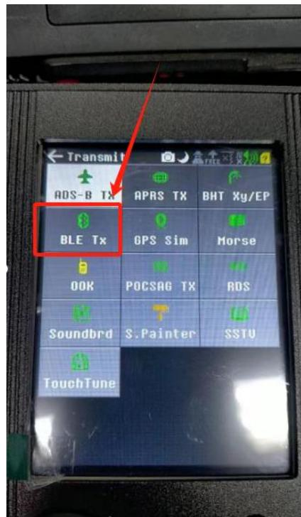
Step 4, transmit the BLE signal. Click the <Open file>, and enter into BLERX file, find <BLE TX Sample.txt>.
