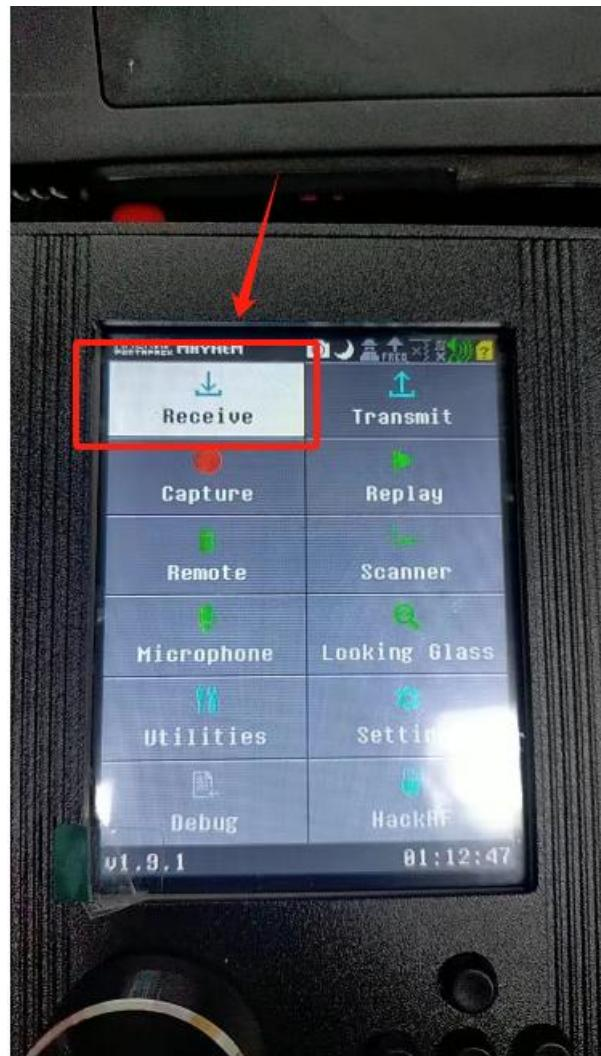
Step 3, click the BLE Rx , enter into the BLE icon, then you will enter into the BLE receive function.
