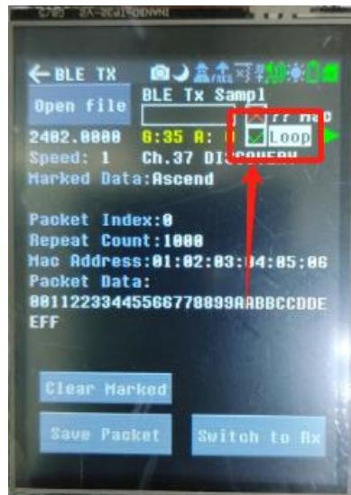
Step 5, click the transmit icon to send the BLE signals (one click the center button of these five buttons when your cursor move to the following icon). Then the device will transmit the BLE signal. You need to one click the center button of these five buttons to stop the transmitting.
