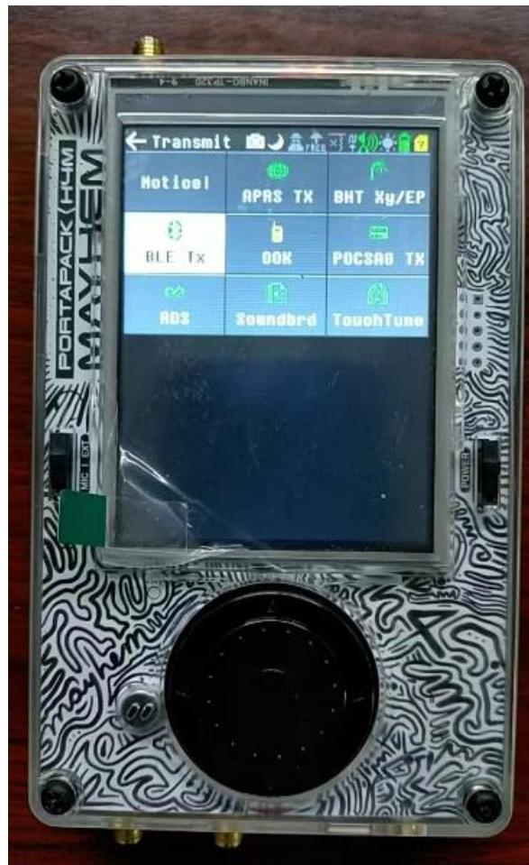
Step 3, click the BLE Tx , enter into the BLE icon, then you will enter into the BLE transmit function.
