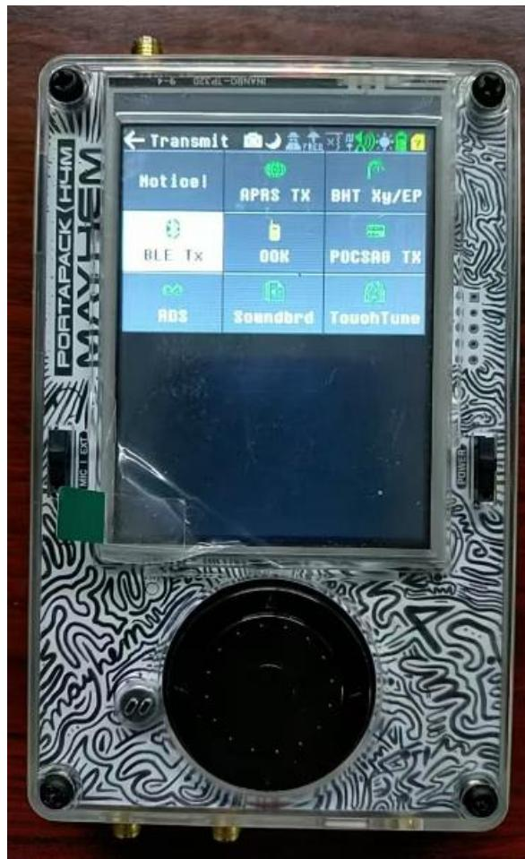
Step 4, transmit the BLE signal. Click the <Open file>, and enter into BLERX file, find <BLE TX Sample.txt>.
