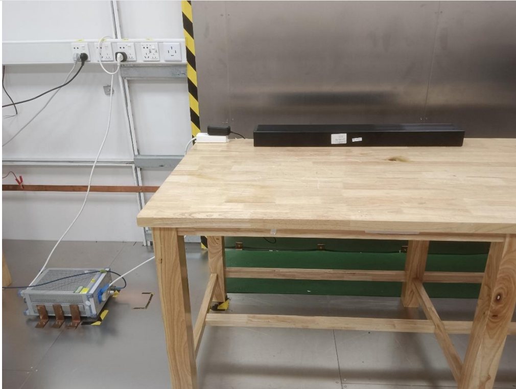
AC Power Line Conducted Emission
