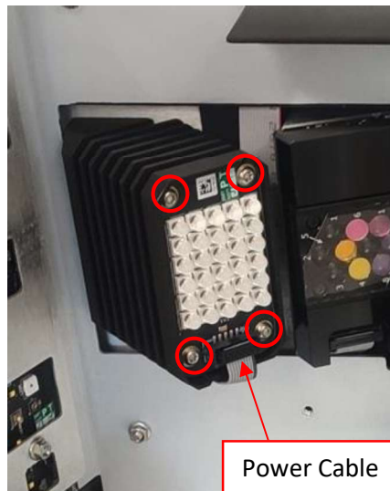
Fig. 24 – 4x (T10 Torx) Anti-stokes PCB retaining screws.
