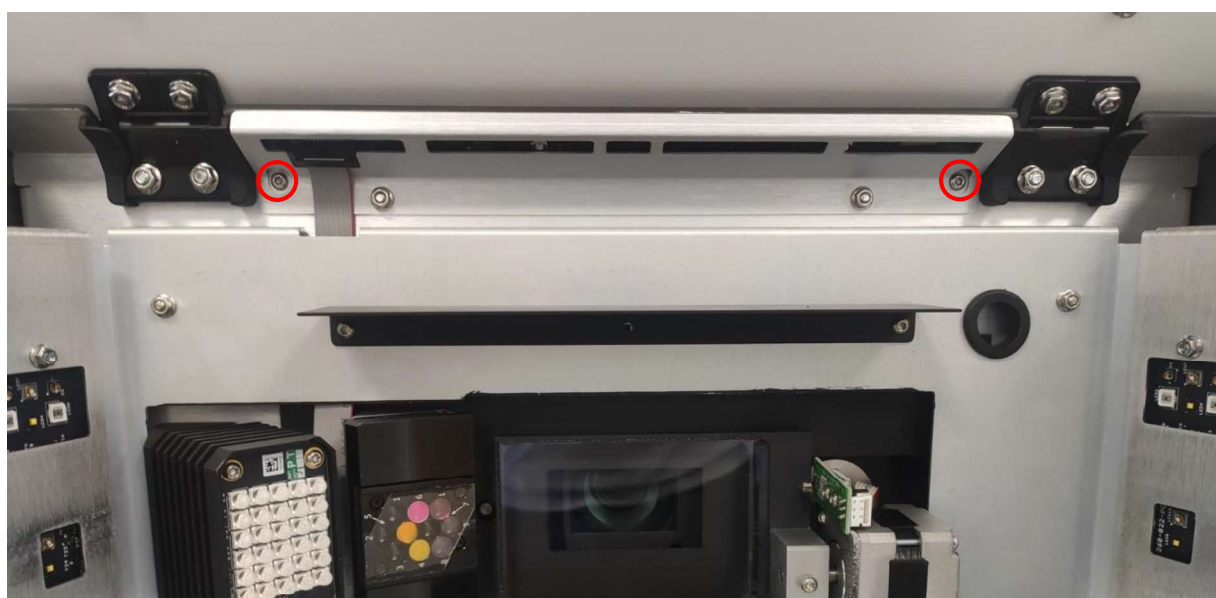
Fig. 3 – 2x (T10 Torx) screws from inside front flap
