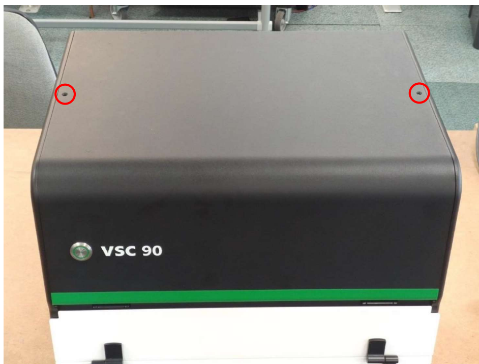
Fig. 1 – 2x (T10 Torx) screws from the centre of the top cover
