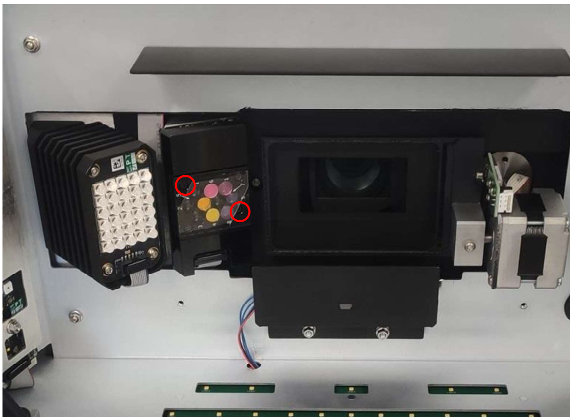
Fig. 30 – 2x (T6 Torx) spotlight array retaining screws.
