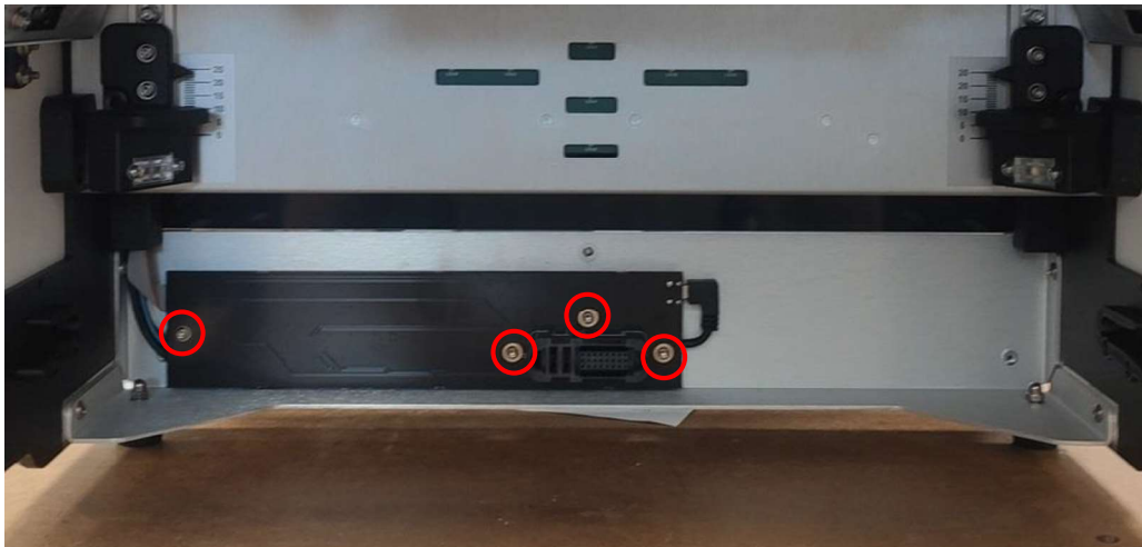
Fig. 34 – 4x (T10 Torx) retaining screws on Backplane Frame PCB
