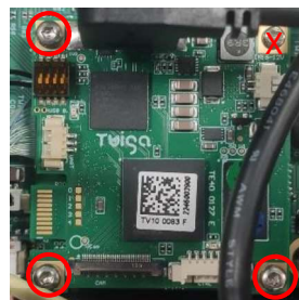
Fig. 19 – 3x (T8 Torx) Interface PCB retaining screws.
