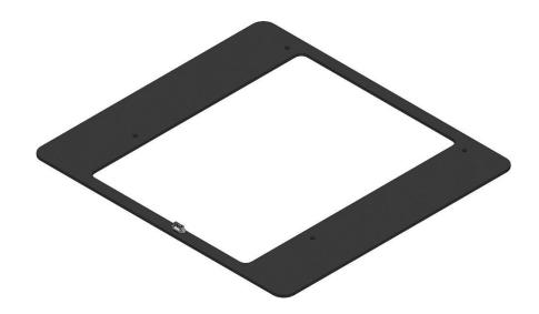
The 284-024-AS RFID Antenna is a differential push/pull input design, which has been designed for use in combination with Advanced Card Systems Ltd.'s ACM1552U-Y3 Driver PCB. The Driver PCB uses a NXP PN5190 NFC driver IC. Connection between the driver and antenna is made via a 5-way Molex Picoblade connector.
