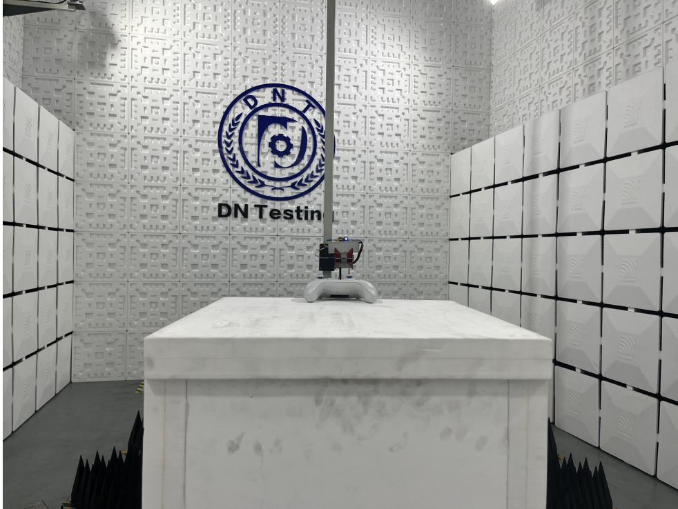
Radiated Emission Test View|(Above 1G)
