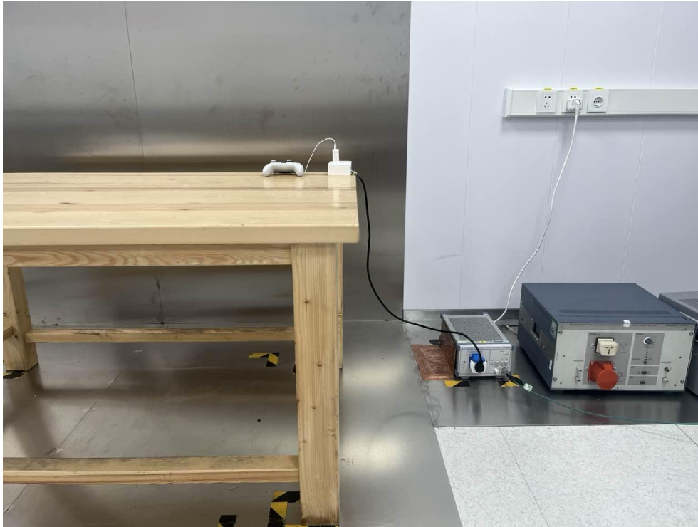
Radiated Emission Test View|(Below 1G)
