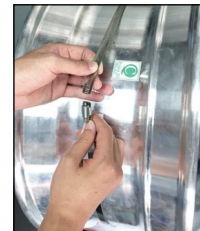
① The steel tie around the hub
