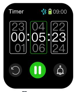
In the picture above, tap the button of to make the timer make no sound when it expires. Slide the number to select the specific countdown length, and then tap the button to enter the countdown page, as shown in the picture below:
