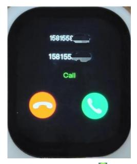
If you want to make a call on the device, tap the button on the Left-side column, or tap the button "Telephone" on the Full Function List Page, and you will be shown the following Telephone Page on which you can slide from left to right to return to the previous page or click the Side Button to return to the Clock Face Page.
