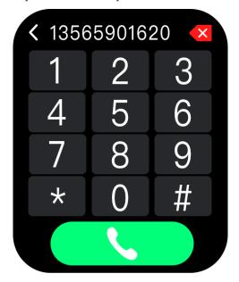
It should be noted that if you cannot make an outgoing call, please check whether the device and mobile phone are connected via Bluetooth and whether the Call Audio Switch is turned on.
