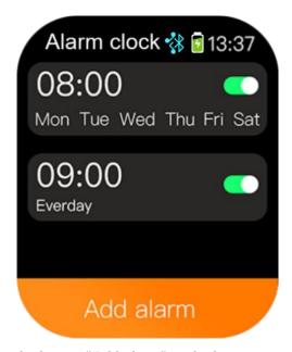
In the picture above, tap the button "Add alarm" at the bottom to add a new alarm clock, or tap one alarm clock (e.g., 08:00 as above) to enter the modification page. You can also tap the switch on the right side of the alarm clock to turn off / on the alarm clock.
