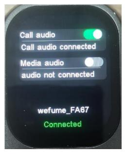
In this case, although you can use the device to make calls, it cannot play music. When the phone and device are already connected via Bluetooth, you need to manually turn on the media audio switch.
