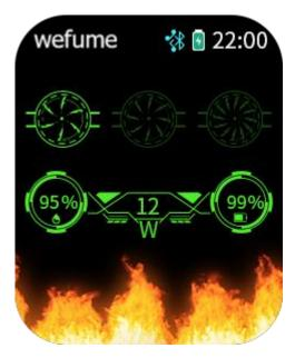
On the Smoking Page, the three gear buttons denote three kinds of power mode for smoking, 12W, 20W and 24W, respectively. The left number 95% shows that there is 95% of e-liquid in the cartridge, while the right number 99% shows 99% of remaining battery capacity and the middle number 12 means the lightest power mode of 12W.
