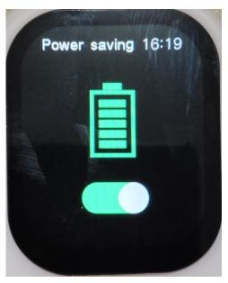
In the picture above, if you turn on the switch, the screen will turn off the highlight mode and the screen brightness will become darker to save power.
