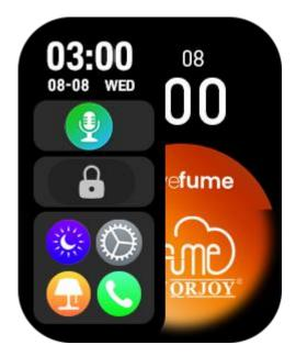
To close the Left-side Column, slide from the right edge of the screen to the left, tap a function item on the Left-side Column, or click the Side Button.
