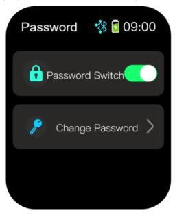
In the picture above, tap "Password switch" to turn the switch on or off. If the switch is turned on, the password protection mode will be activated and a password will be required to input as shown in the picture below:
