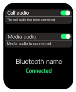
As can be seen from the picture above, both the Call audio switch and the Media audio switch are turned on. What's more, on some frequently used function pages, there is an icon on the upper edge of the screen to indicate that the call audio switch has been turned on, as shown in the red box in the figure below.
