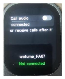
To do this, you need to manually turn on the call audio switch in the picture above to allow the device to connect to the mobile phone via Bluetooth. Then refer to Step 2 for help.
