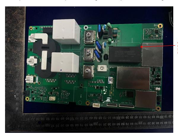
Optional power module 1 Model: RAC20C-12SK/277 Supplier: RECOM Rating: 100-277VAC
