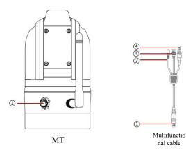
Multifunctional cable (1): Connect to the interface of the infrared MT thermal imager (1), and align the white dot on the power cord end with the white dot on the device before insertion.
