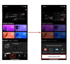
Power on the camera and open WLAN in Settings. Select the Wi-Fi name of the dome camera and enter the password. By default, the Wi-Fi name is MT\_xxxx (xxxx indicates the device type and SN) and the password is 12345678.
