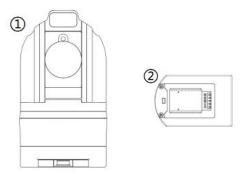
Install battery ② to the bottom of the ①MT. After the battery is installed,, press and hold the power button on the battery for a few seconds to start supplying power to the device and turn it on.
