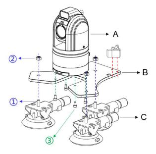
There is 1 camera (A), 1 base (B), 3 suction cups and some screws ( $\mathbb{D}(2)$ 3). First, fix those parts together as shown in the figure above. Next, fit the dome camera with suction cups and place it properly on the roof.
