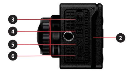
④ Type-C 3.0 OTG Port (for connecting to a computer for data transfer and UVC function)
