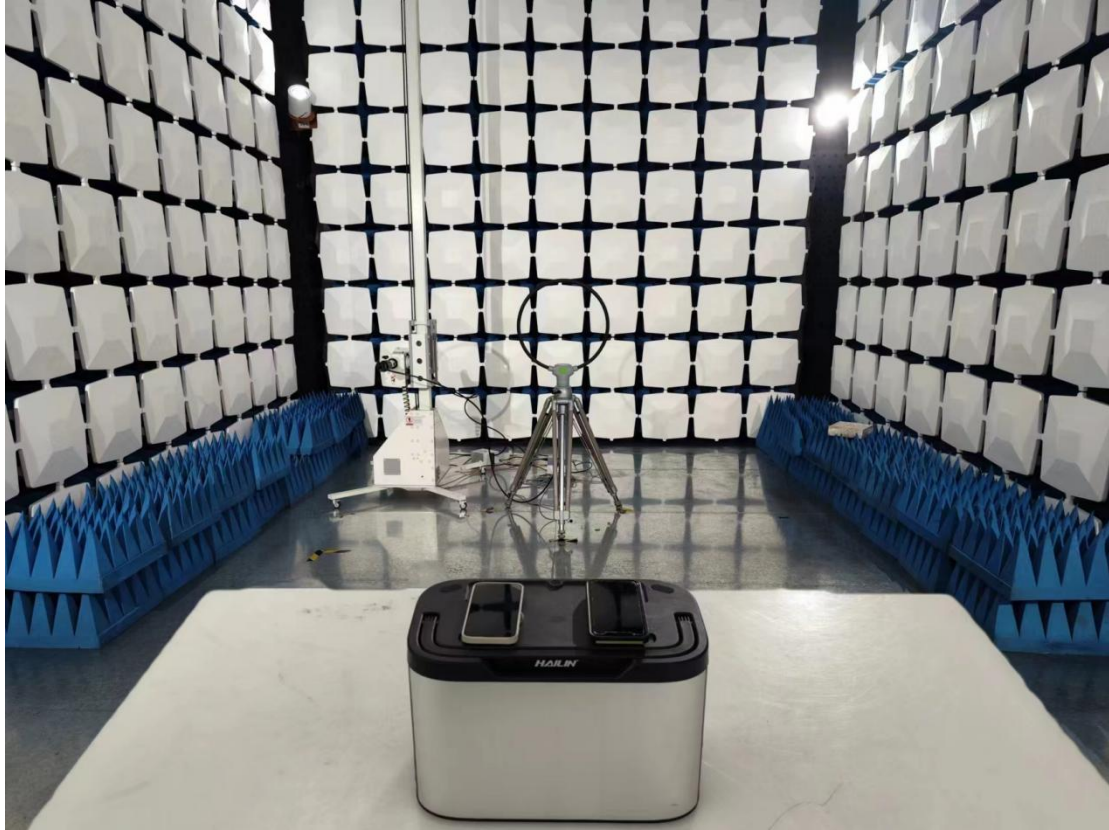
Blow 1GHz for radiated emission test setup
