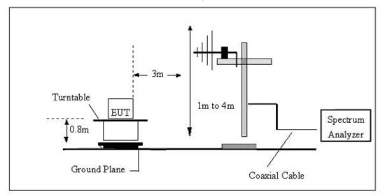
(C) Radiated Emission Test-Up Frequency Above 1GHz
