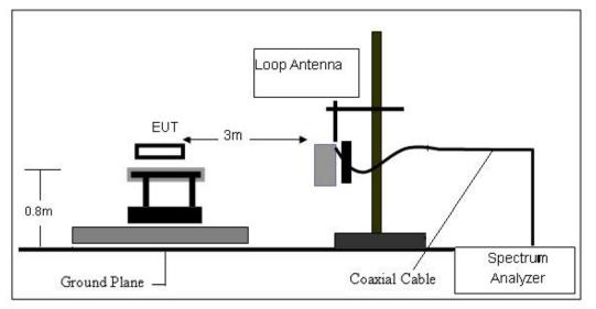
(B) Radiated Emission Test-Up Frequency 30MHz~1GHz
