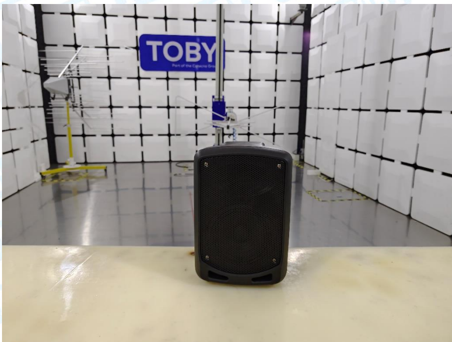
Photo of Setup for Radiated Emission (30MHz~1GHz)
