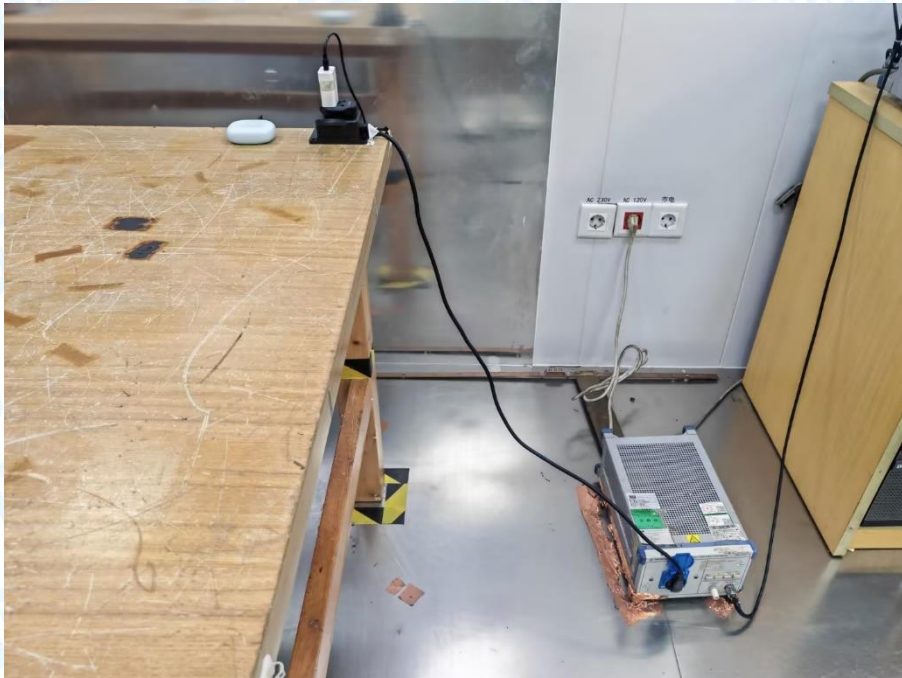
Photo of Setup for Radiated Emission (30MHz~1GHz)
