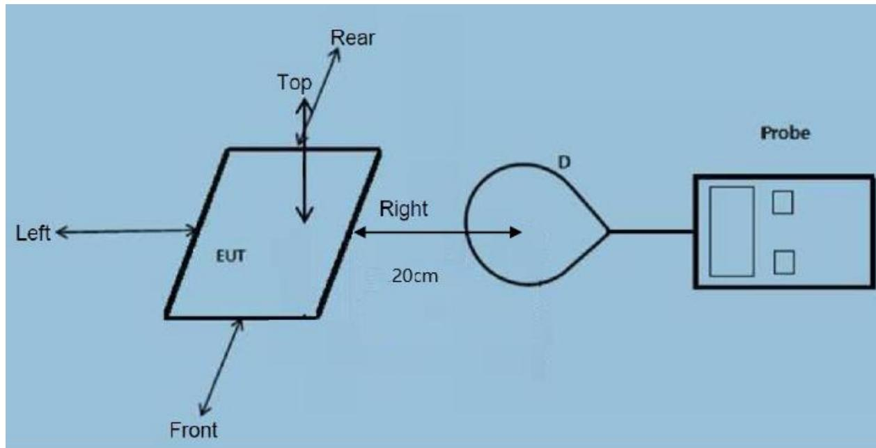
Note: Measurements should be made from all sides and the top of the primary/client pair, with the 20cm measured from the center of the probe(s) to the edge of the device
