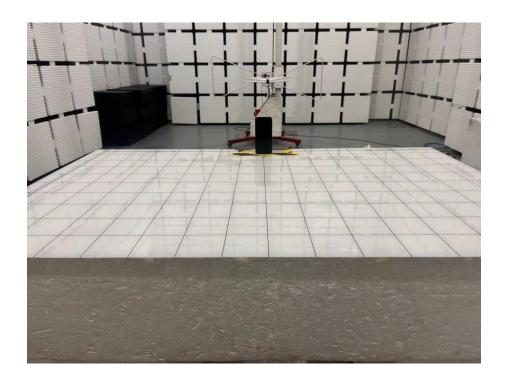
Set-up for Radiated Spurious Emission, Above 1GHz
