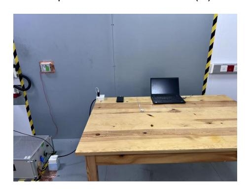
Set-up for Radiated Emission (RE), Below 1GHz
