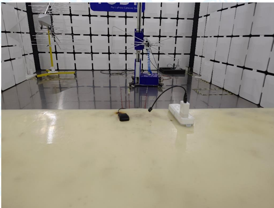
Photo of Setup for Radiated Emission (30MHz~1GHz)
