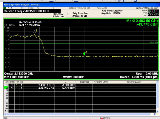
Out Of Band Emission(Right) 8DPSK_3-DH5_Channel Hopping
