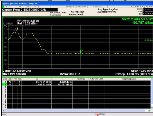
Out Of Band Emission(Right) GFSK_DH5_Channel Hopping
