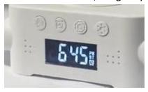
Remark: Short press to increase 1 hour or 1 minute, long press to adjust hours and minutes rapidly.
