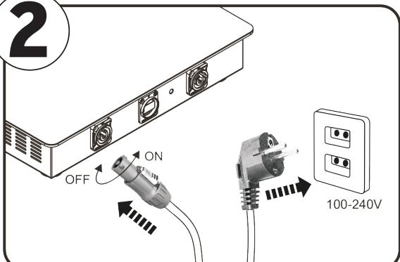
INSERT THE BLUE PLUG OF THE WIRE INTO THE BLUE SOCKET OF THE BASE, TURN RIGHT IS "ON" AND TURN LEFT IS "OFF".
