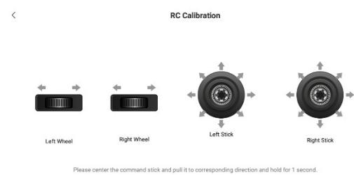
Please center the command stick and pull it to corresponding direction and hold for 1 second.
