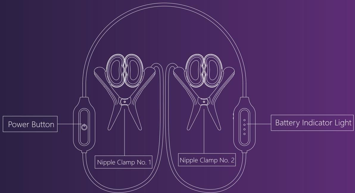
**Switch Control:** Press and hold the power button for 1.5 seconds to power on or off. After powering on, the button indicator light and battery indicator light will illuminate simultaneously.
