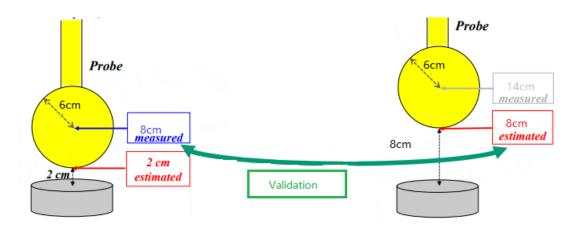
2.By calculation, the percentage of estimated H-field value at a distance of 2cm from the EUT coil on the surface of the probe sensor=(estimated H-field value (8cm)) - actual measured H-field value (8cm))/estimated
