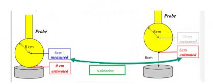
1. By calculation, the percentage of estimated H-field value at a distance of 0cm from the EUT coil on the surface of the probe sensor=(estimated H-field value (6cm) - actual measured H-field value (6cm))/estimated H-field value (6cm) \* 100%; The estimated percentage of the E-field at a distance of 0cm from the EUT coil on the surface of the probe sensor=(estimated E-field value (6cm) - actual measured E-field value (6cm))/estimated E-field value (6cm) \* 100%
